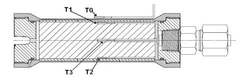
Figure 1. Instrumented Sub-scale Cookoff Chamber (propellant charge 45.7 mm diameter x 114.3 mm long)
