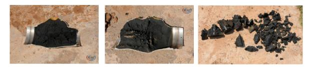
When tested in composite cases, the XLDB propellants demonstrated the ability to achieve no reaction to fragment impact velocities up to 2530 m/s (Figures 8 and 9). Additional testing is planned to explore variables in grain design and their impact on fragment impact performance.
