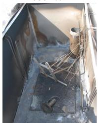
The SCO testing performed under this study serves to demonstrate that this family of minimum smoke propellants can pass SCO without secondary autoignition devices. The motor geometry chosen was selected to represent the typical size and configuration of tactical ground-launched or aviation-launched propulsion systems.
